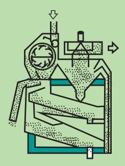
At the last leg in the process, through the Sortex machine, we make sure yellow or black kernels of rice do not get mixed with the final product. The final rice has to be white in colour.
